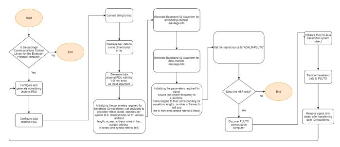
Figure 7: Transmitter Flowchart
