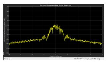
Figure 10: Received Spectrum When Packets Are Being Transmitted, Calculated PER = 0.125523
