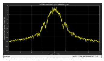
Figure 11: Received Spectrum When Packets Are Being Transmitted, Calculated PER = 0.098522.
