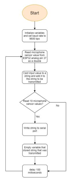
Figure 5: Flowchart Displaying the Functionality of Microcontroller
