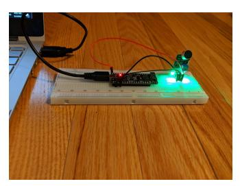
Figure 4: Connection of LM393 Microphone with ESP32-PICO-KIT Microcontroller
