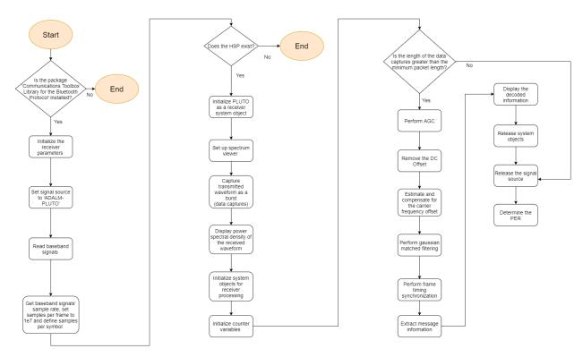
Figure 8: Receiver Flowchart
