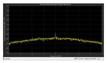
Figure 9: Received Spectrum When No Packets Are Being Transmitted
