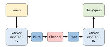
Figure 2: Block Diagram of the Overall Design's Data Transmission Path
