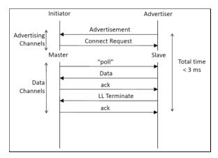
Figure 1: Overview of BLE Communication System
